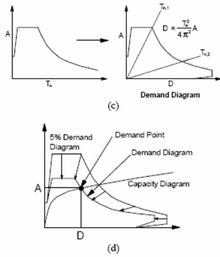
(c) conversion of elastic response spectrum from standard format to A-D format, (d) determination of displacement demand
