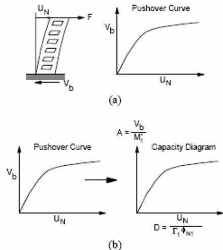
CSM: (a) Pushover curve, (b) Conversion of pushover curve to  $q_3$  capacity spectrum
