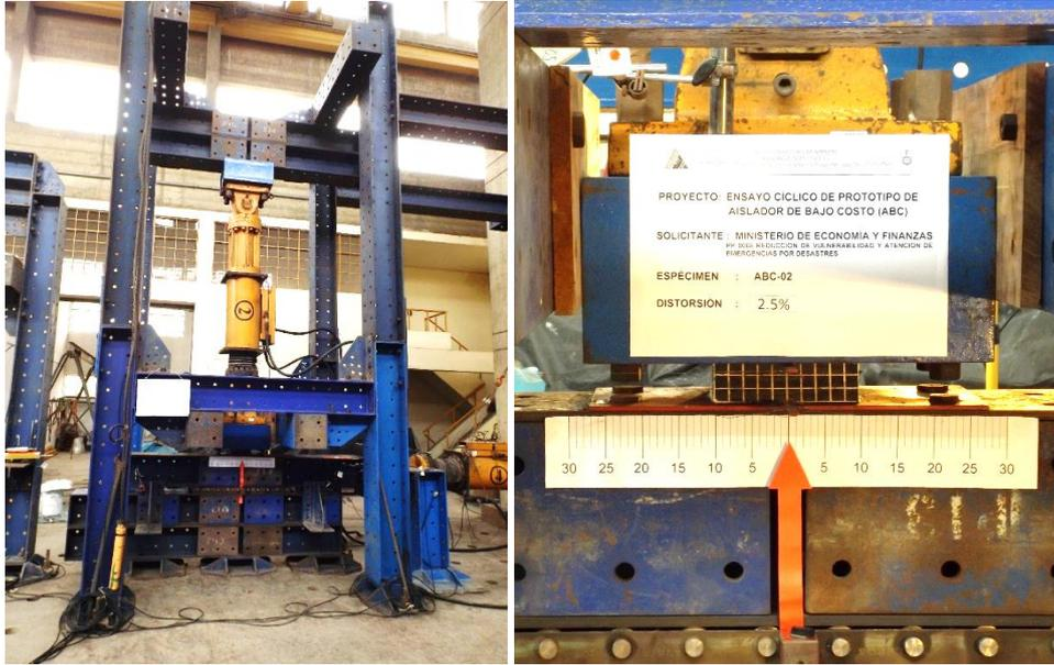
Fig. 6 – Loading frame and specimen
