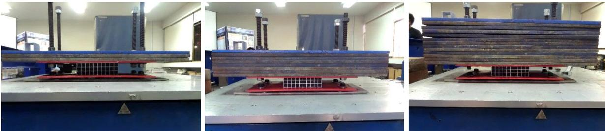
Fig. 2 – Free vibration test with different dead load applied
