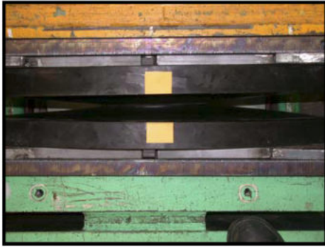
Figure 5: RoGlider ready for testing Displacement 0mm – Load 850kN
