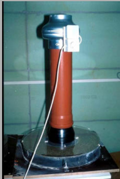
Testing crack formation due to drying shrinkage
