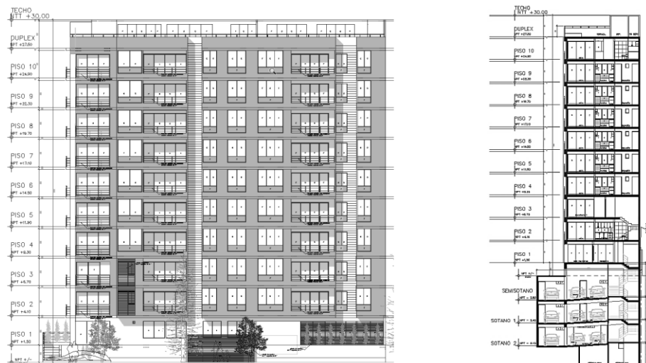
Fig. 2 – Front Elevation (left) and Transversal Section (right) of the 1 ST Peruvian Building
