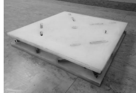
Seismic Isolator composed of linear rails TRC15
